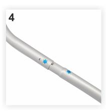
3. Once all the aluminium tubes provided with elastic are joined, you will get: four straight bars (for the vertical sides of the PopUp) and four curved bars (for the horizontal sides of the PopUp).
